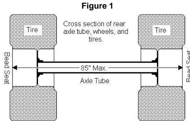
The maximum overall width of a Supermodified shall be 85 inches measured from the left, outer bead seat to the right, outer bead seat. This includes all portions of the car. No allowances. (see figure 1) No fan cars, boxing, tunneling, or ground effects are allowed. No body panel of any material shall be extended below or outside of the lower frame rails on all four sides of the Supermodified.
